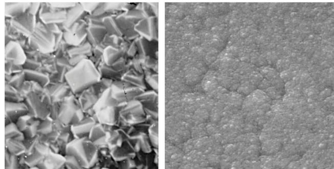
**Fig. 1 — Contrasting the difference between the surface of a PCD die (left) and a Nano-Die (right) at 4000x magnification.**
