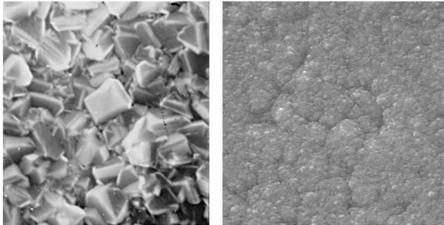
**Fig. 2 — PCD surface (4000 times magnification) (left) and Nanocrystalline Diamond surface (4000 times magnification) (right).**
